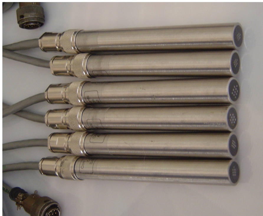
Figure 3. Typical coupled multi-electrode array sensor probes used in the experiments.
