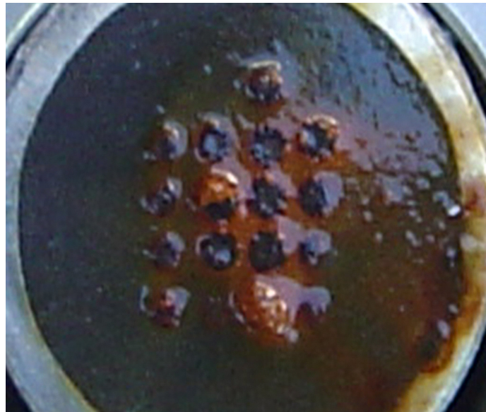
Figure 7. Appearance of the CS 1008 probe immediately after removal from the simulated seawater, after the corrosion rate measurement.
