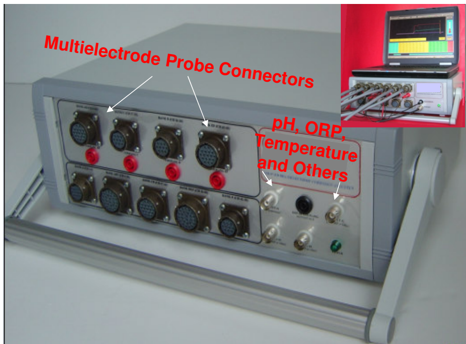
Figure 2. Coupled multi-electrode analyzer used in the experiments and typical real-time displays on a notebook computer (see insert).
