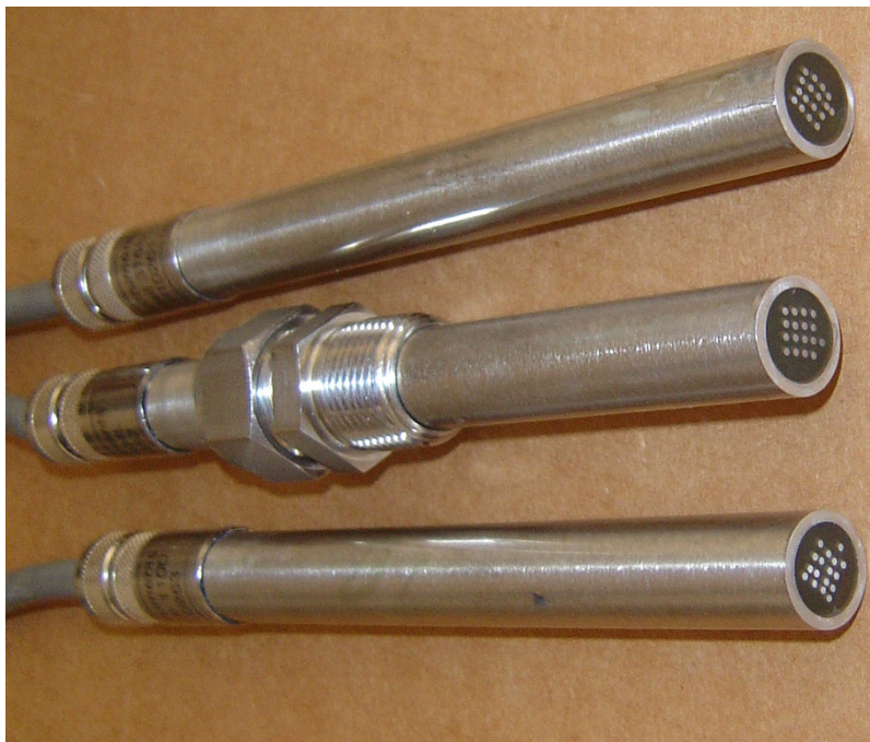
Figure 2. Typical coupled multielectrode array sensor probes.
