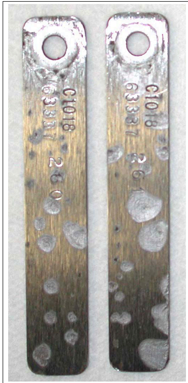
Figure 13: Field Corrosion Coupons after 1-month exposure in plant water. (Note that the areas outside of the under-deposit corroded locations still show the machining lines of the coupons from fabrication suggesting that once under-deposit corrosion initiated, corrosion propagated rapidly in these areas)
