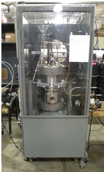
Figure 1: 20L high pressure autoclave used in this study
