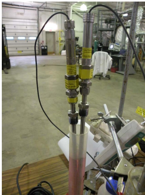
Figure 3: High pressure glass pH probe and Ag/AgCl reference electrode used to measure proton (hydronium ion) concentration.
