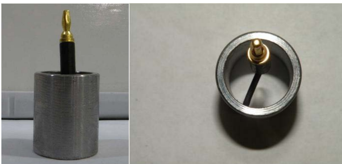
Figure 1: Specimen for HPHT rotating cylinder electrode
